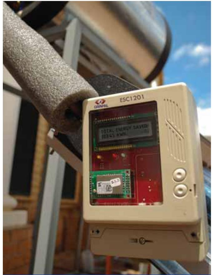
*Above: SWH energy measurement device (ESC 1201)*
