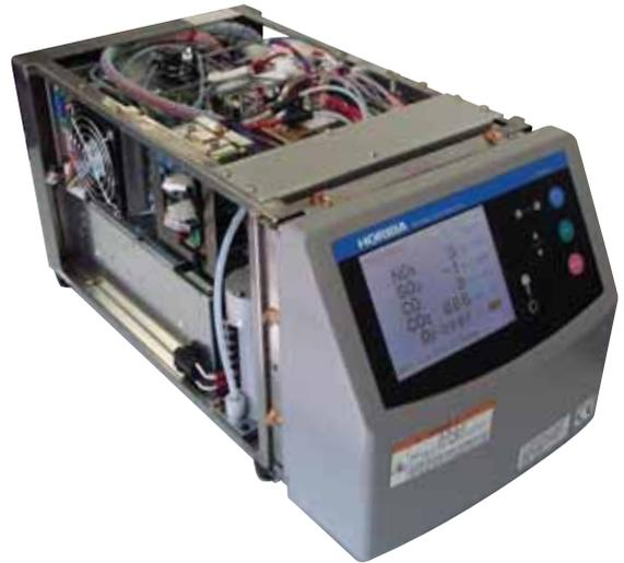
The PG250 provides the user with an interface which indicates actual, live conditions within the stack, i.e. gaseous concentrations, so the industry is able to make informed adjustments to their systems to improve their processes, and so reduce their emissions and their impact on the environment.
